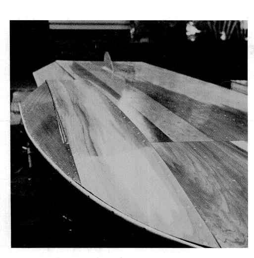
18. Front view of the finished sponson; the correct angle of the sponsons and workmanship at this point will mean a lot in the handling of WETBACK.
