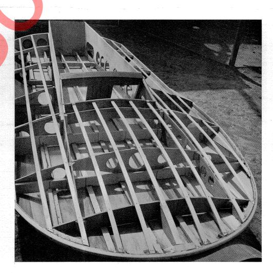
14. Construction view prior to any decking. Position of dashboard was later changed; it was moved about 8" towards the transom, as in the plans. The edges of the deck battens were rounded a bit where fabric would lay, for a smoother fit. Better placement of the lightening holes were made in the plans for rib #2.
