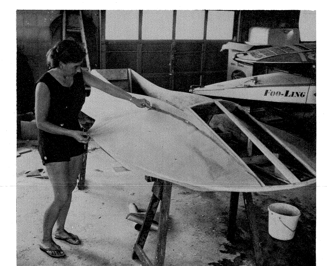
22. Jupiter ready for planking, try to get the deck battens to take a nice smooth curve from transon to rib #5, and at rib #5 has a 45° cut out that the rest of the bottom which also has a 45° cut will overlap at rib #5.
