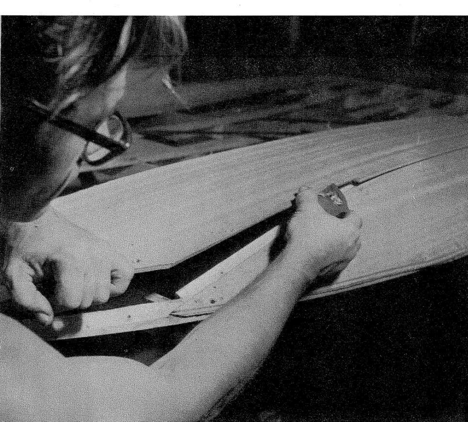
15. Here the spinnaker planking has been fastened in place, and carefully trimmed. See rib drawings and notice how the side of the bottom has a lip more the back of the spinnaker.
