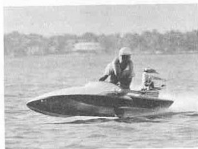
Most popular hydro class is the 20 cubic inch B Stock. Three point hulls are generally used. Note the two forward sponsons free of the water.
