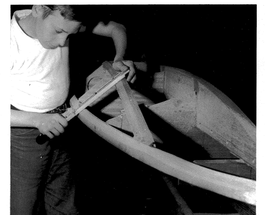
24. Bow piece and sponson chine are carefully faired. The sponson chine is made up of two \frac{1}{2} " thick pieces of spruce.
