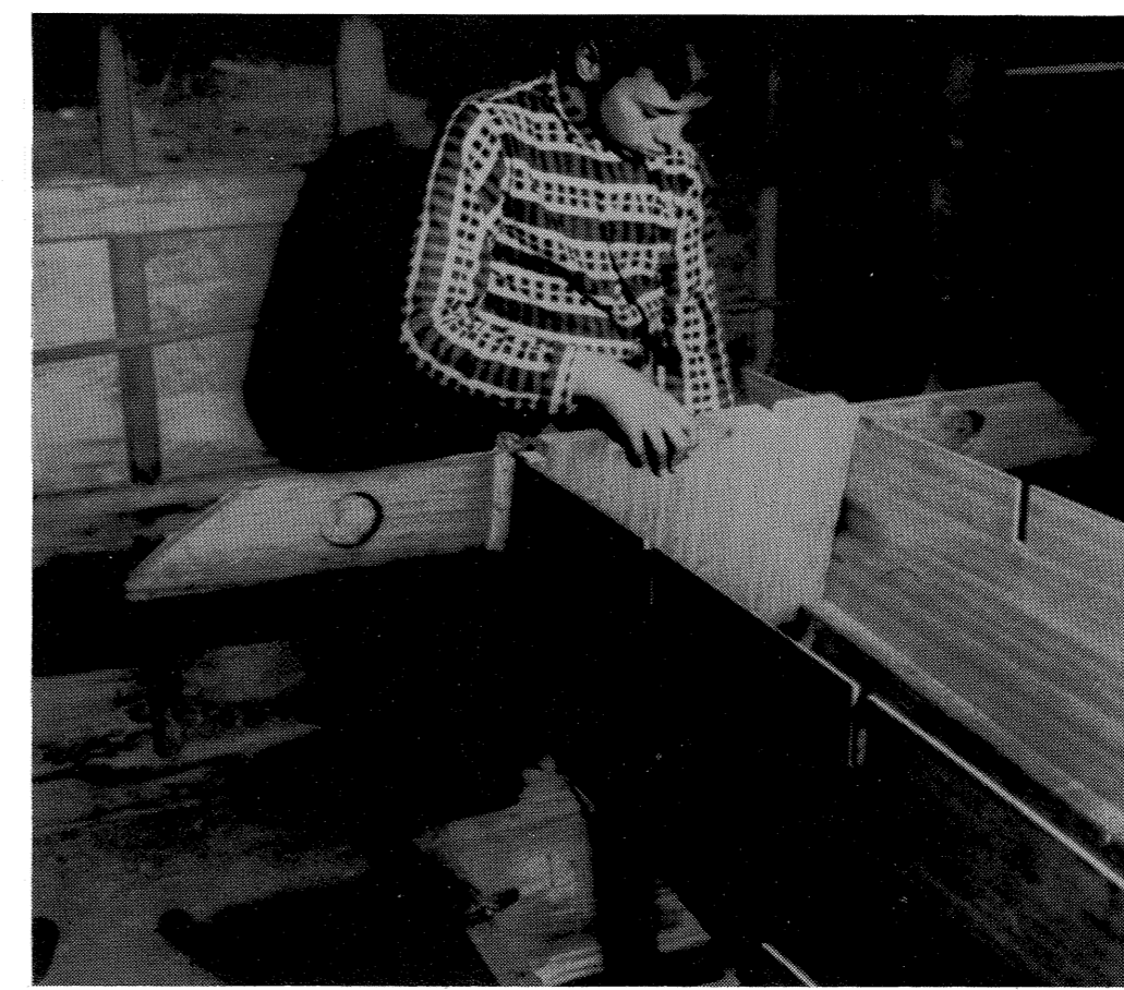
5. Girders are set up on a simple jig 18" apart and rib #8 is secured. Then the motor mount is placed in front of rib.
