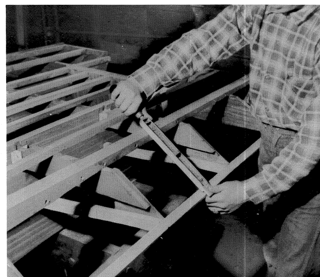
19. Chine and sheer are carefully faired with a wood file prior to planking.
