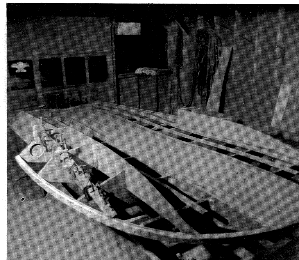
22. The center section batten tapers to nothing between rib #1 and #2.
