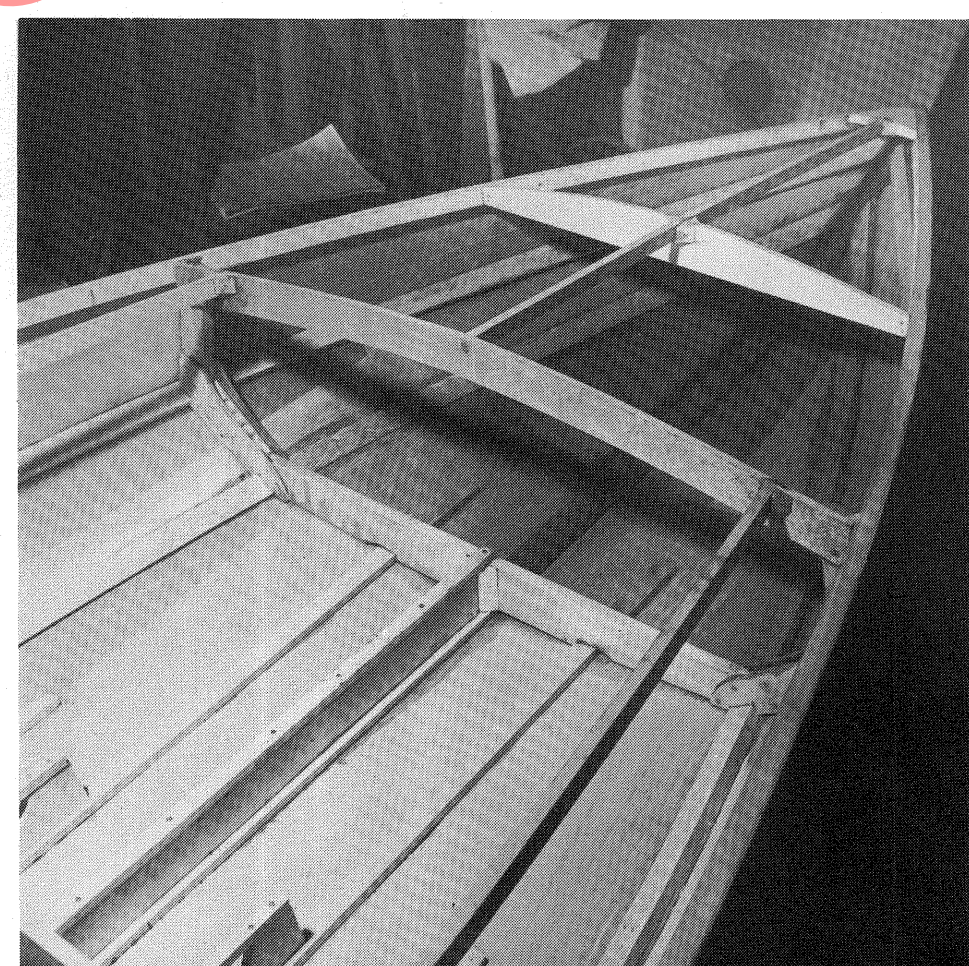
14. Bow complete ready for decking, under deck I have already given 4 coats of varnish, a lot easier than when the deck is on.
