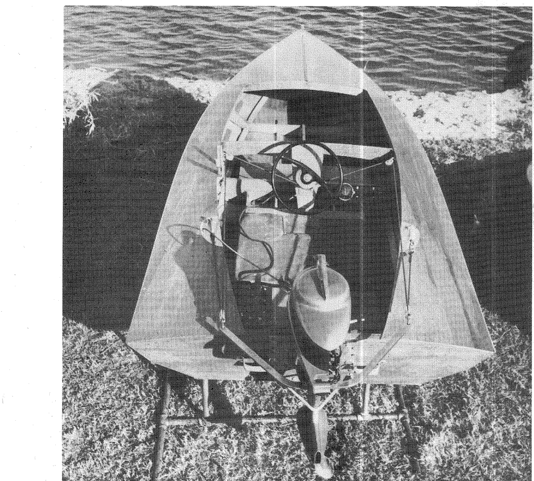
5. AIRBORNE all set up, ready to race. Note cut down Mercury tank that fits between the stringers of the boat.
