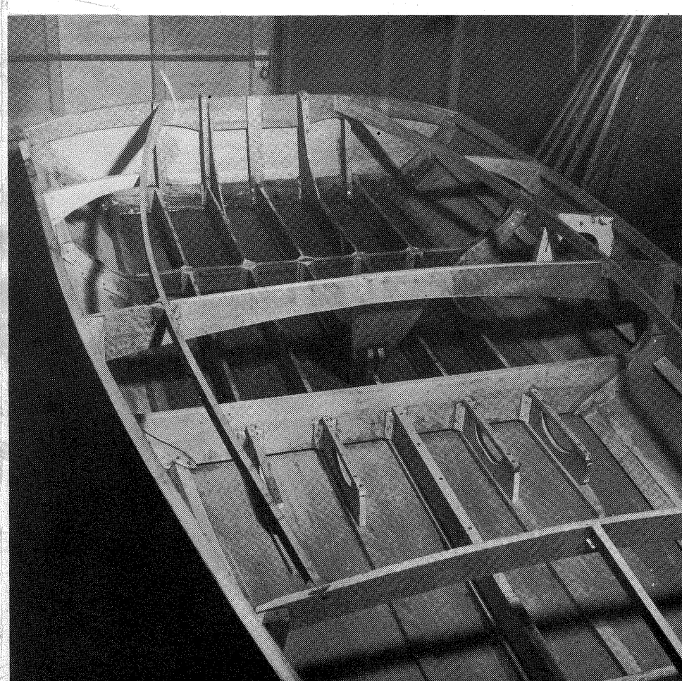
15. This picture should answer a lot of questions. The bottom is glued up and with Anchorfast nails to all battens. About 8" on center.
